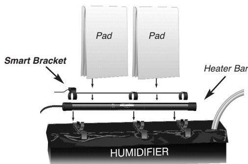
For use with H-5 Humidistat. Eliminates uncertainty as to when to change humidifier pads. When humidifier pads dry out and no longer wick water, the red SB light, marked PADS, blinks. The SB shuts off the humidifier heater bar so it will not dry the piano when the humidistat is calling for moisture.
