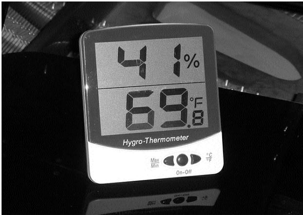
Simultaneously displays temperature and humidity on jumbo LCD panel. Designed for desk display or wall mounting.
