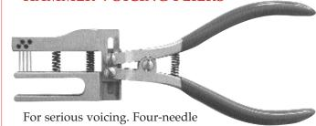
parallel-action pliers are applied to side of hammers, softening the inner portions of the hammer, while leaving outside tension intact. Same as used in upscale piano factories. Particularly effective for opening up tone in treble section. Length is 8½".
